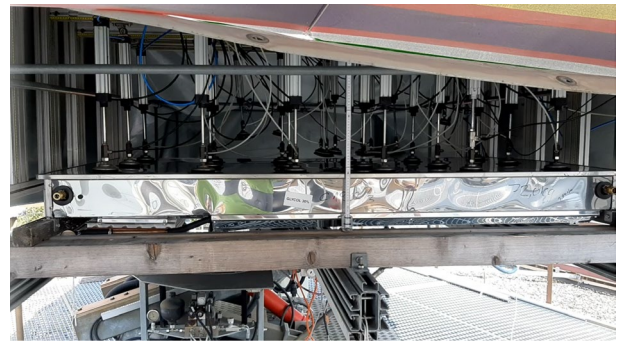
Figure 11: Positive mechanical load test (snow)
