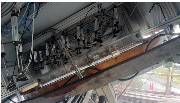
Figure 10: Negative mechanical load test (wind)
